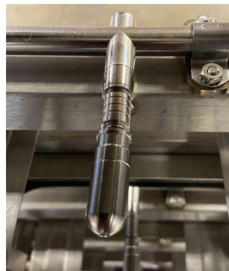
Lane Shur-flo valve, Quick connect and manifold installed on rack
